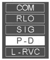
Select the P-D function and confirm by pressing the OK button. The device will go into the PD testing mode and display the following information:
