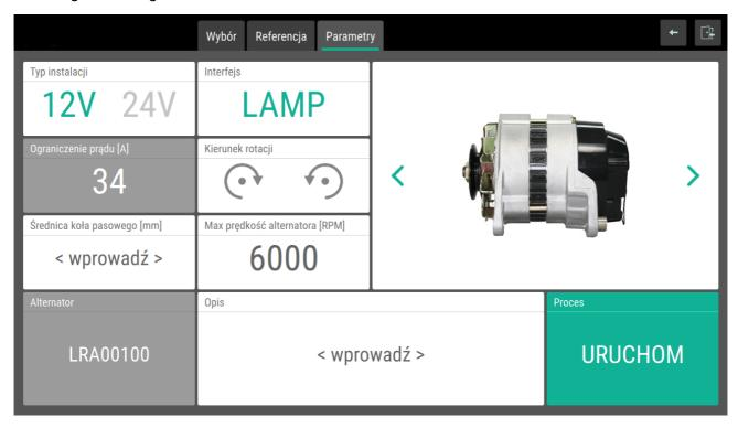
The next stage is selecting detailed parameters of the test. In most events the parameters are downloaded from the database, however in case some information is unavailable in the database or user considers it as an invalid it is possible to change such parameters as:
