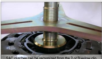
SAC clutches can be recognized from the 2 or 3 yellow clip placed on the mechanism.
