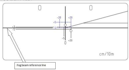
Check the position of the low beam projection on the aiming screen match the reference lines
