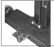
The optical chamber is adjustable in height by means of slides on precise, silent, plastic runners on a column marked with a centimeter scale for exact positioning with respect to the headlight.
