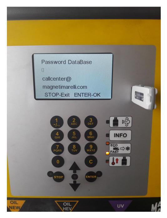
3. After switch on device appeared comunicate <u>Password Database</u> should write password from service Magneti Marelli Aftermarket. Password is generating on base serial number of device. Nameplate is stick on back side of device <u>Serial N°</u>
