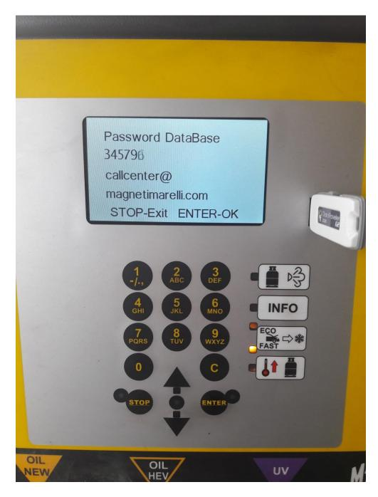
5. Received password should write and confirm push button: Enter.
