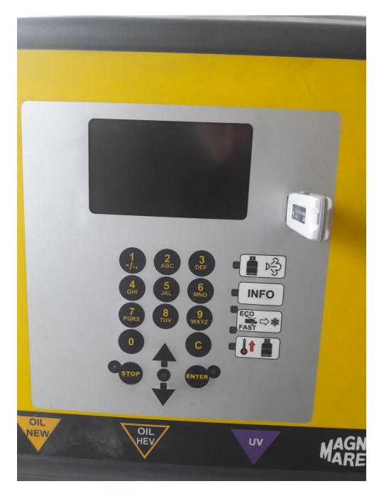
2. After received new database, copy file <u>36-cardb.dta</u> (data base on refigerent r134a) or file <u>33-cardb.dta</u> (data base on refigerent 1234yf) on empty Pen drive, and put it to port USB in front display of device. Switch on device in back side of device.
