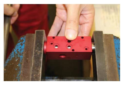
5. Put the o-rings on the bottom of the valve (greased with technical vaseline) and tighten the valve back to the pump. Connect the air hose.
