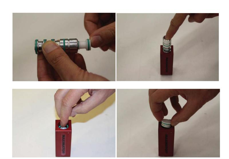
4. Install a new Seger's ring and then adjust the appropriate guide sleeve to push it in place (eg with a vice).
