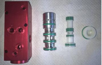
3. Clean all parts of the valve (with f.e. extraction gasoline), check o-rings (if they are worn, replace them) and during assembly lubricate parts, especially o-rings, with f.e. technical Vaseline
